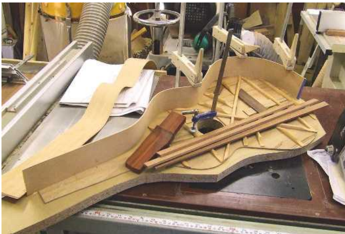
▲ Pic.16 Remove excess on the top with a bandsaw. A dry-fit will ensure you find gaps before getting the glue out!
